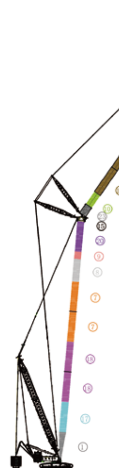
超起塔式副臂 Superlift tower jib SHW: (48-96)+(30-102)m
